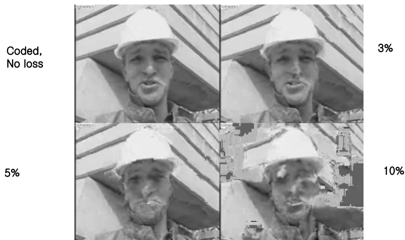
Example: reconstructed video frames from a H.264 coded sequence, subject to packet losses
